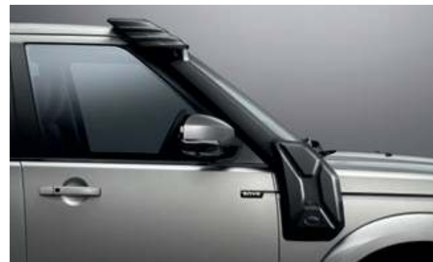
Raised Air Intake VPLAP0018
