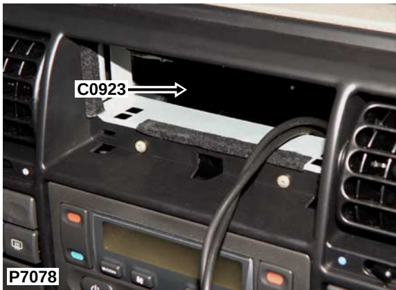
Description: Head Unit-Audio System Location: Behind radio
