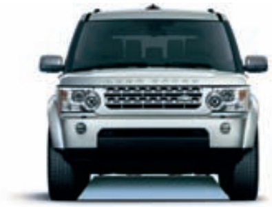
Obstacle Clearance Ground clearance off-road height up to 9.5 inches/240mm, with air suspension raised Standard ride height 7.28 inches/185mm
