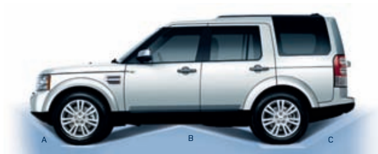
A Approach Angle Standard ride height 32.2° Off-road ride height 37.2°, w/air suspension raised
