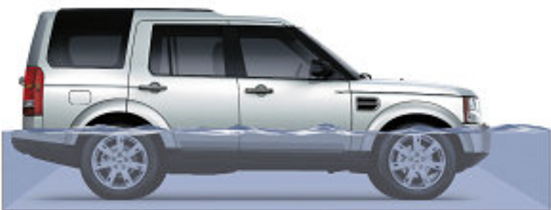
Wading Depth Maximum wading depth 27.6 inches (700mm) (in off-road mode)
