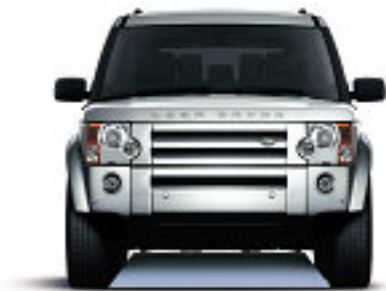
Minimum Ground Clearance Ground clearance up to 9.5 inches (240mm) (air suspension) Standard ride height 7.3 inches (185mm)
