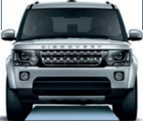
Obstacle Clearance Off-road height up to 310mm Standard ride height up to 185mm
